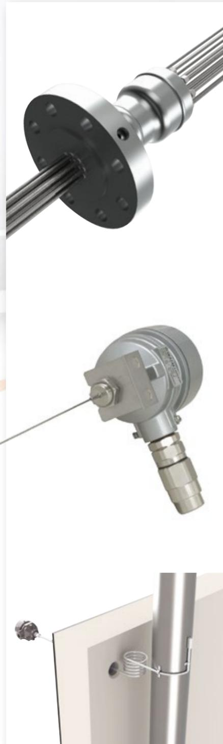
OMC's extensive range of electric heating systems is constructed using the company's own manufactured mineral insulated cables. This manufacturing process offers ease of installation, since the sheath can be supplied to a bend radius of 2.5 times the heater OD. This means the heater can be formed into any desired shape and is high pressure sealed for welding when required into process flanges.
