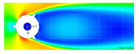
Have a look at the image from the same independent report by Cygnet Development Systems – showing the velocity plot of the flowrates around an Okazaki Vortexwell Thermowell which clearly demonstrates that the design greatly reduces vortex induction.
