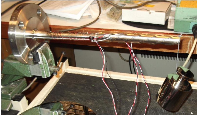
Figure 7 Preliminary Strain Measurement for Validating FE Meshes
